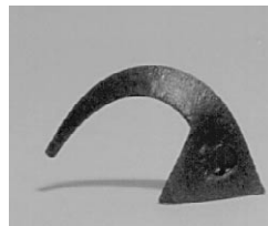
A perfect bend. Do not be concerned if the cone bends a little higher or lower than this one.
