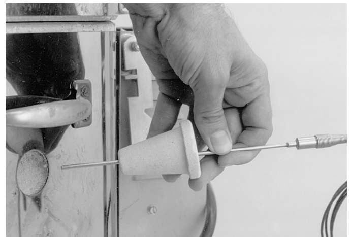
Using a drilled peephole plug to attach the thermocouple to the kiln. Make sure the thermocouple does not fall out of the kiln.
