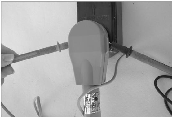
Checking the voltage under load (while the kiln is firing).
