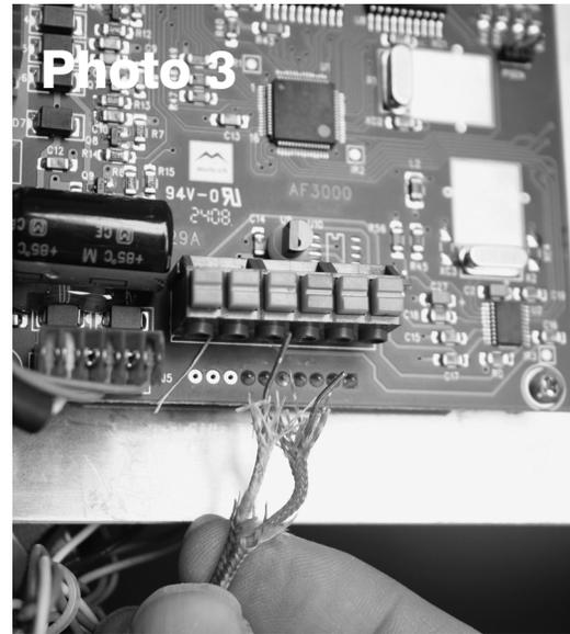
The 2 thermocouple wires are connected to the bottom of the controller. After reinstalling, tug on the wires to make sure they are secure.
