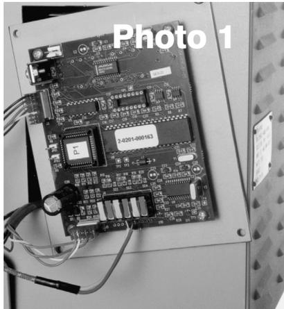
Remove the 4 corner screws and turn the controller over so the back is facing you.
