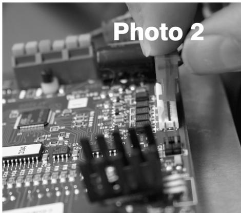
Remove the 2 wire connection plugs. When reinstalling, do not force the plugs.
