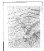
Front Loading Kilns: The element must fit all the way into the back of each firebrick corner. These elements are not pre-bent for the corners. However, bending the element for
