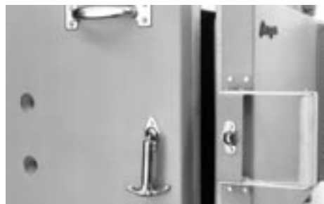
Tapered peepholes offer a wide view. The spring-loaded door latch helps hold in the heat.
